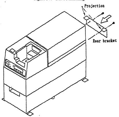
Figure 1-8. Rear Bracket Attachment
